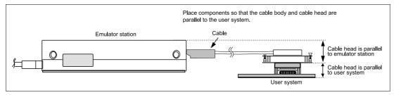
Figure 10 User System Interface Cable Location Example
